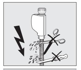
Do not cut or damage the inlet hose in any way.
